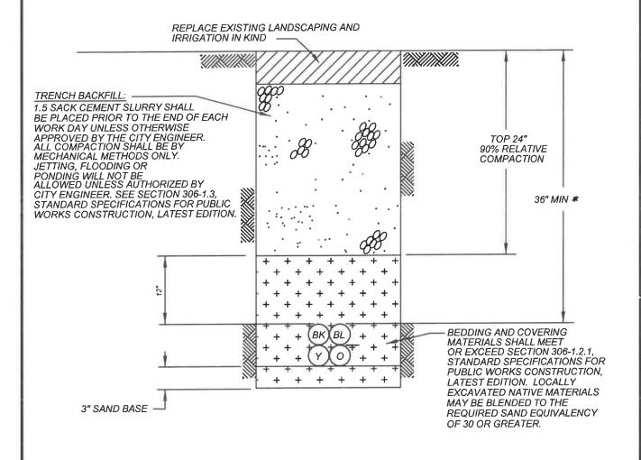
\* 36" MIN FOR TRUNK AND DISTRIBUTION CONDUIT SYSTEM AND 18" MIN. FOR SERVICE LATERAL CONDUIT SYSTEM.
