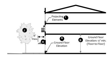
Note to Staff: floor-to-floor measurements were used because this is a constant, while ceiling heights may be changed easily by tenants
