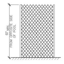
MESH SIZE FOR CHAIN LINK FENCES SHALL BE NOT GREATER THAN 2 1/4" SQUARE UNLESS THE FENCE IS PROVIDED WITH SLATS FASTENED AT THE TOP OR BOTTOM WHICH REDUCE THEOPENINGS TO NOT MORE THAN 13/4"
