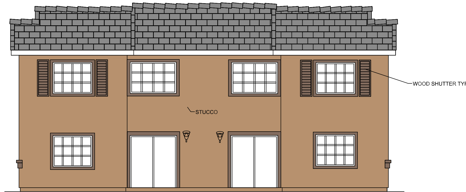
REAR ELEVATION (ROOF TYPE "B") (DUPLEX) 1" = 6'-0"
