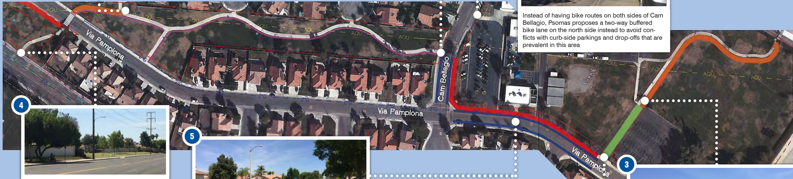
4 A high visibility crosswalk, Rectangular Rapid Flashing Beacon (RRFB) and refuge islands are recommended to aid pedestrians and cyclists to cross at this location. The two-way cycle track being recommended should reduce crossing distance for pedestrians and cyclists.
