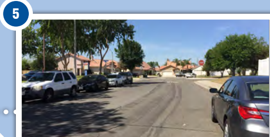
5 Instead of having bike routes on both sides of Cam Bellagio, Psomas proposes a two-way buffered bike lane on the north side instead to avoid conflicts with curb-side parkings and drop-offs that are prevalent in this area
