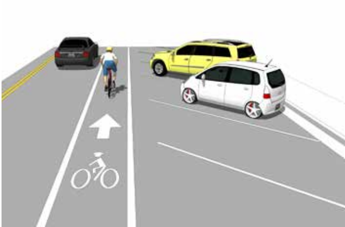
10B) Reverse angled parking greatly improves visibility of oncoming traffic, including cyclists, for vehicle drivers exiting parking stalls
