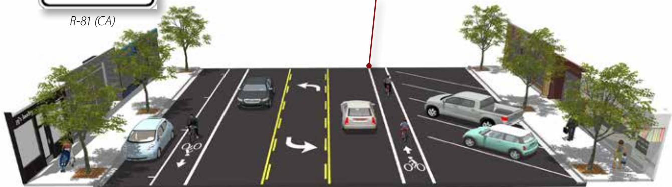
Bicycle lane with back-in/head-out angle parking
