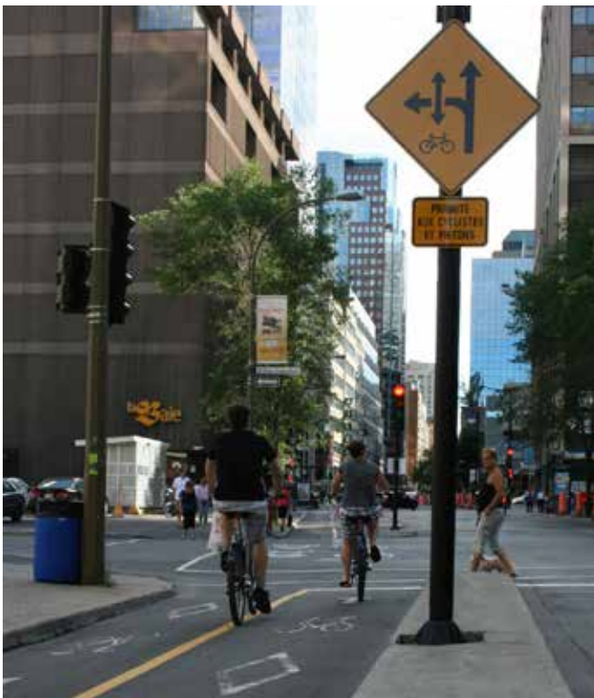
Cycle track (Signage informs left-turning vehicle drivers that cyclists and pedestrians have priority) - Montreal, Quebec
