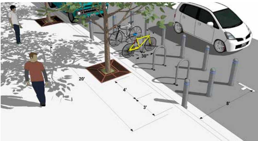
Bicycle corral dimensions - Converts one car parking space into 8-10 bicycle spaces
